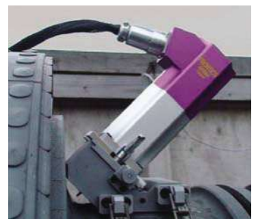
▶ Testable exclusively attached to the Rotor Groove
